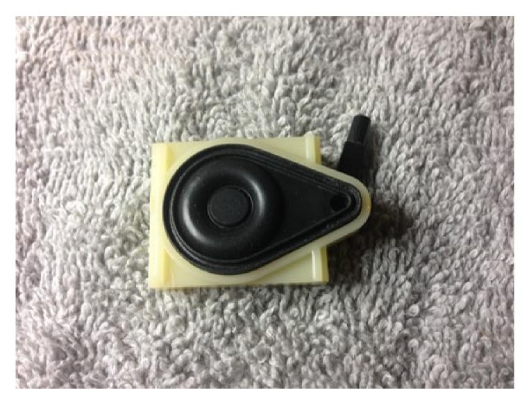
This is the other side of the bladder. It is sealed by the bottom of the BC2 case.
