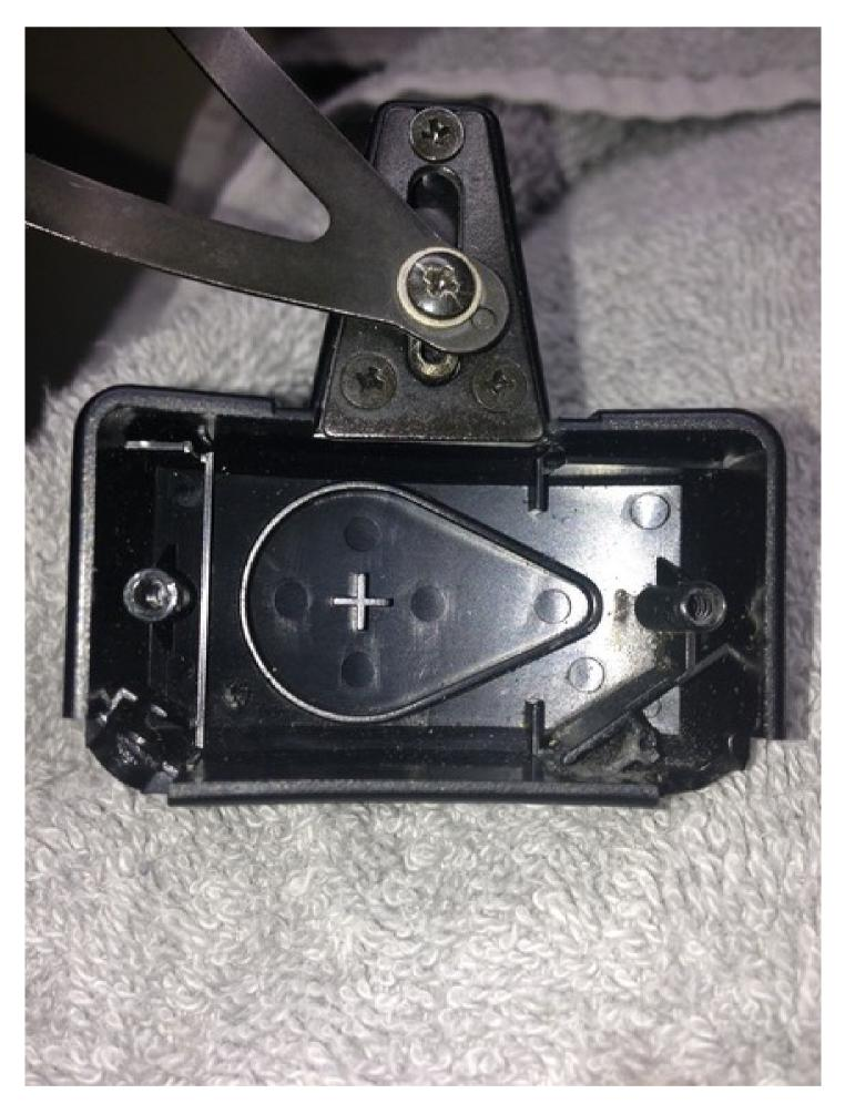
This is the inside of the headpiece showing where the PCB sits. The teardrop shaped feature seals the rubber bladder while the "+" in the center preloads the rubber bladder so it sits close to the hall effect sensor on the PCB.
