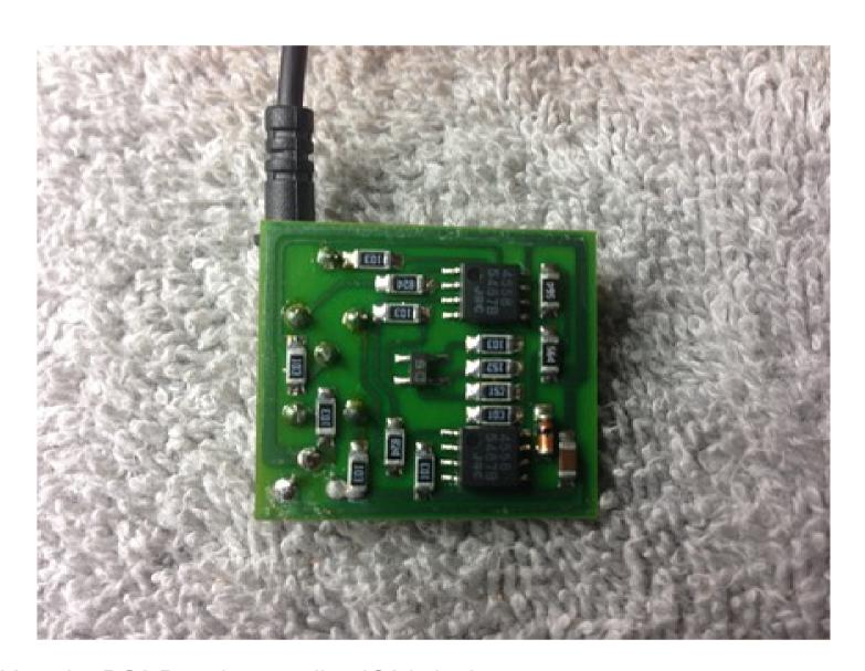
Component Side of Yamaha BC2 Breath controller. IC3 is in the very center and is a hall-effect sensor which increase it's output as the magnetic field above it is increased.
